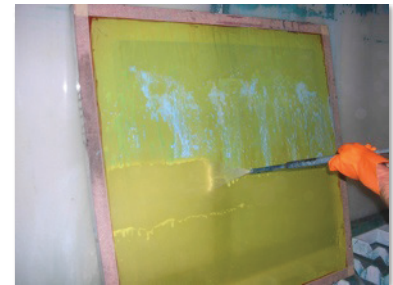
Step 3. High pressure rinse - starting at bottom.
