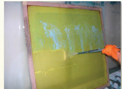
Step 3. High pressure rinse - starting at bottom.
