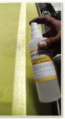
**Step 1**. Apply an even layer of instant adhesive, using the applicator tip provided, to the surface to be bonded.
