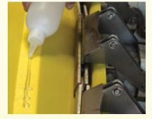
Ste p 1. Apply an even layer of instant adhesive, using the applicator tip provided, to the surface to be bonded.
