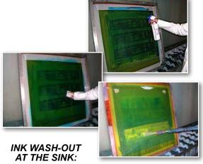
Card excessive ink from the screen. Apply **ECO-STRIP**® to ink side of screen. Use a non-abrasive scrub brush or pad to agitate ink on both sides of screen. Finally, rinse away all all residue away using high pressure water.
