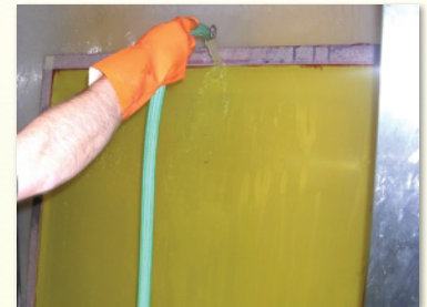
3. Flood rinse the screen starting at the top and washing all residue off the screen.
