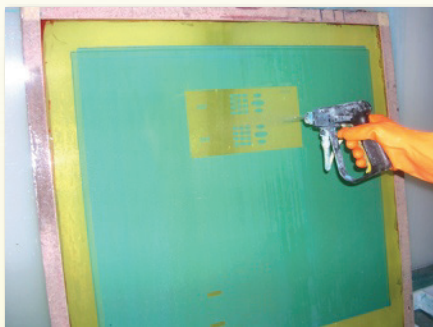
Step 1. After removal of ink, block-out, and tape, apply ER/35® to a wet screen (both sides).
