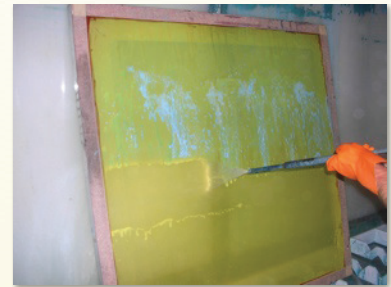
Step 3. High pressure rinse - starting at bottom.
