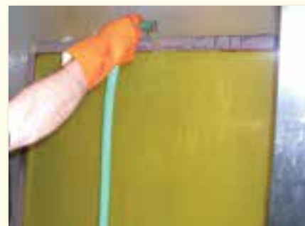
3. Flood rinse the screen starting at the top and washing all residue off the screen.
