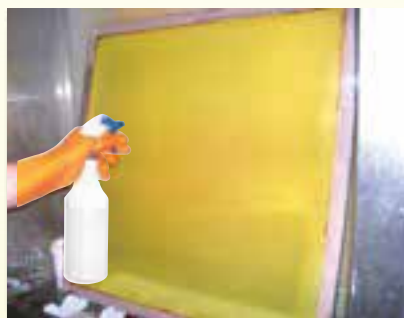
1. After removal of ink, block-out, and emulsion, spray FAB-90 to the screen(both sides).
