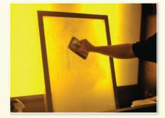
Step 2. Scrub screen with non-abrasive pad or brush. Allow screen to sit for up to 10 minutes.
