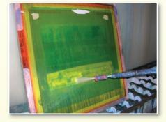
**Step 3.** High pressure rinse the screen starting at the bottom. Reverse screen and high pressure rinse. Continue washing off any blockout that remains.
