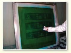
**Step 2.** Scrub screen with a non-abrasive pad or brush until all ink is completely liquified.
