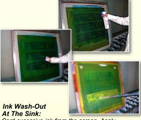
Card excessive ink from the screen. Apply IW-18 to ink side of screen. Use a non-abrasive scrub brush or pad to agitate ink on both sides of screen. Finally, rinse all residue away using high pressure water.
