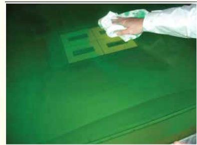
Step 3. Use rags or towels to wipe up ink residue. Re-apply to clean up ink residue in image area.
