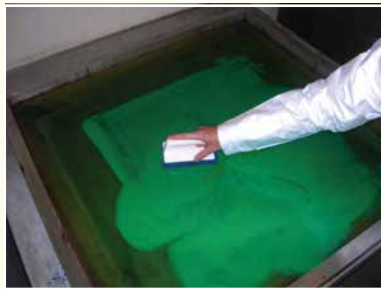
Step 2. Scrub ink with a non-absorbent pad until liquified.
