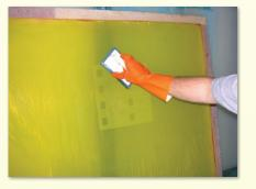
**Step 2.** Scrub screen with non-abrasive pad or brush. Allow product to sit on screen for up to 10 minutes.
