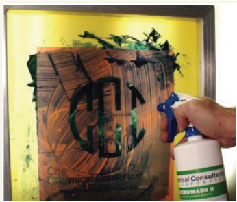
Step 1. After removal of ink, and tape, apply MicroWash II to a wet screen(both sides).
