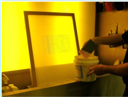
Step 1. Apply ProChem® AD-606 to both sides of the screen.
