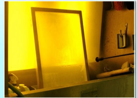
Step 3. High pressure rinse - starting at bottom.
