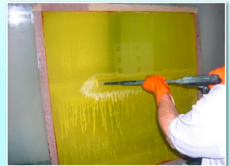
Step 3. High pressure rinse - starting at bottom.
