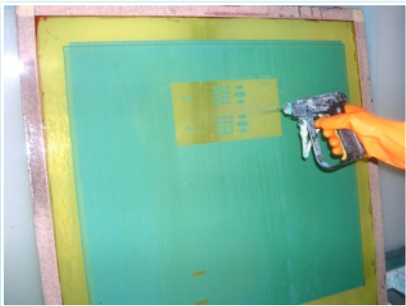
Step 1. After removal of ink, block-out, and tape, apply ProChem® ES-530 to a wet screen (both sides).
