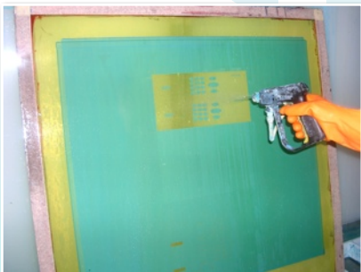
Step 1. After removal of ink, block-out, and tape, apply ProChem® ES-900 to a wet screen(both sides).
