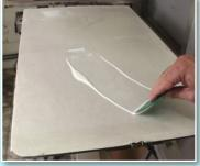
Drop a quarter size amount onto pallet and spread with a plastic spreader or rigid card stock. Cover entire pallet or area large enough to cover print area.
