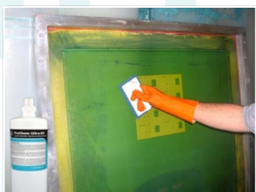
Step 1. Apply Ultra-DX on both sides of the screen. Scrub with a non-abrasive pad or brush.
