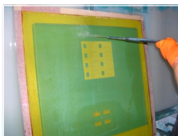
Step 2. Allow Ultra-DX to dwell on the screen for 1-3 minutes. High pressure rinse - starting at bottom.
