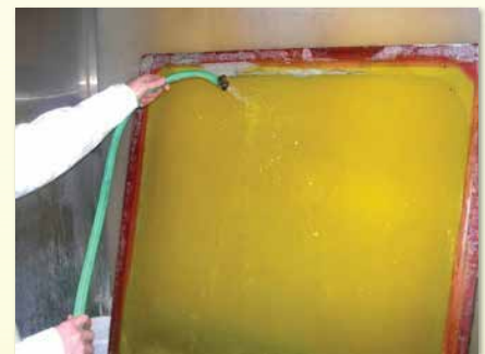
Step 3. Flood rinse the screen starting at the top and washing all residue off the screen.
