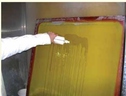
Step 1. After removal of ink, block-out, and emulsion, apply Prep-Rite to the screen(both sides).
