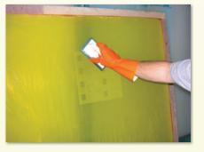
**Step 2.** Scrub screen with non-abrasive pad or brush. Allow screen to sit for up to 10 minutes.
