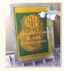
**Step 1.**Spray **RTU** on both sides of the screen.
