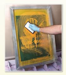
**Step 2.**Scrub screen with a non-abrasive pad or brush until all ink is completely liquified.
