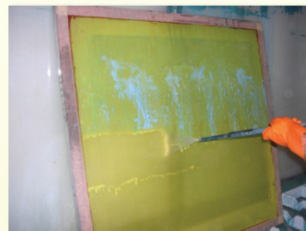
Step 3. High pressure rinse - starting at bottom.
