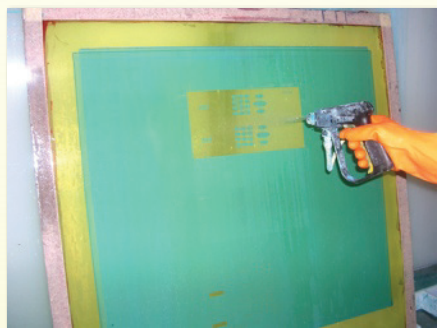
Step 1. After removal of ink, block-out, and tape, apply SMP® solution to a wet screen (both sides).
