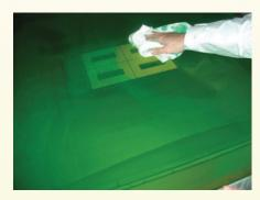
**Step 3**. Use rags or towels to wipe up ink residue. Re-apply to clean up ink residue in image area.
