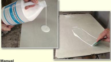
Drop a quarter size amount onto pallet and spread with a plastic spreader or rigid card stock. Cover entire pallet or area large enough to cover print area.
