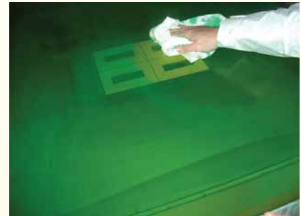
Step 3. Use rags or towels to wipe up ink residue. Re-apply to clean up ink residue in image area.
